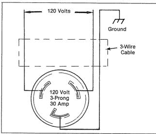
A 120 volt, 3-prong, 30 amp connector plug is included with the alternator. If additional plugs are required, refer to REPAIR PARTS section of manual. A 3-wire cable must be purchased and connected to the plug as shown above.
